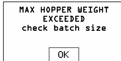
Figure 42: Typical "Maximum Hopper Weight" Alarm Screen
